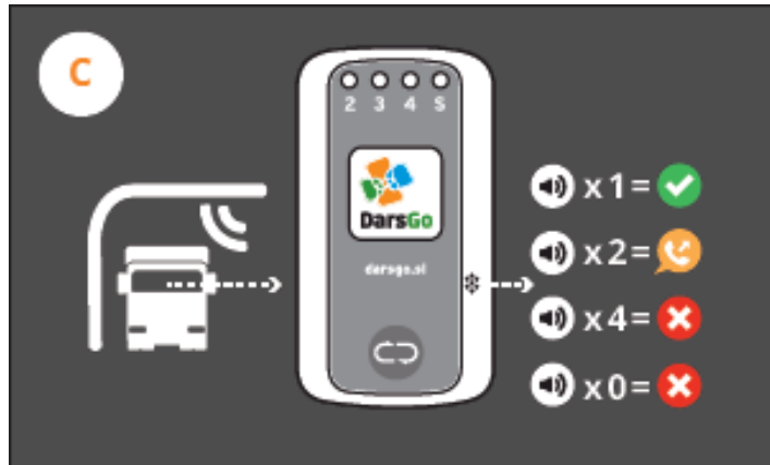
Figure 3: Signals of the DarsGo unit while passing tolling points
