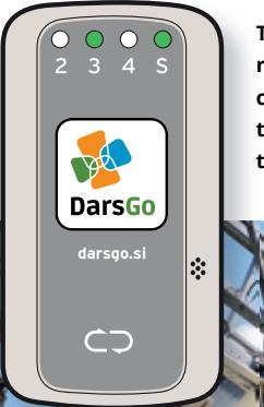
The DarsGo unit will register the vehicle registration number and EURO emission class, and the toll class will be specified by the driver before each trip with respect to the number of vehicle axles.
